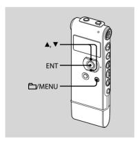
You can erase unwanted messages, retaining all other messages when the IC recorder is in the stop or playback mode. When a message is erased, the remaining messages will advance and be renumbered so that there will be no space between messages.
